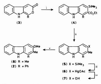
Scheme 1. [Compounds (3)–(7): a, R = Me; b, R = Ph] Reagents: i, EtO<sub>2</sub>CC=CSiMe<sub>3</sub>, PhBr, reflux; ii, LiAlH<sub>4</sub>, dioxane, reflux; iii, Hg(OAc)<sub>2</sub>, AcOH; iv, BH<sub>3</sub>-THF; alkaline H<sub>2</sub>O<sub>2</sub> work-up; v, MeI, K<sub>2</sub>CO<sub>3</sub>, acetone, reflux.
